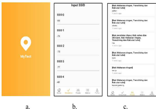
Fig. 5 Application Mockup: a) Splash Screen; b) Received signal from the adjacent SSID; c) Monitoring the other's position
