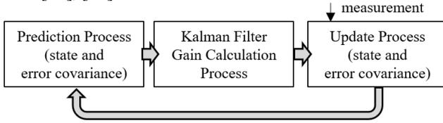
Fig. 1 Kalman filter algorithm
