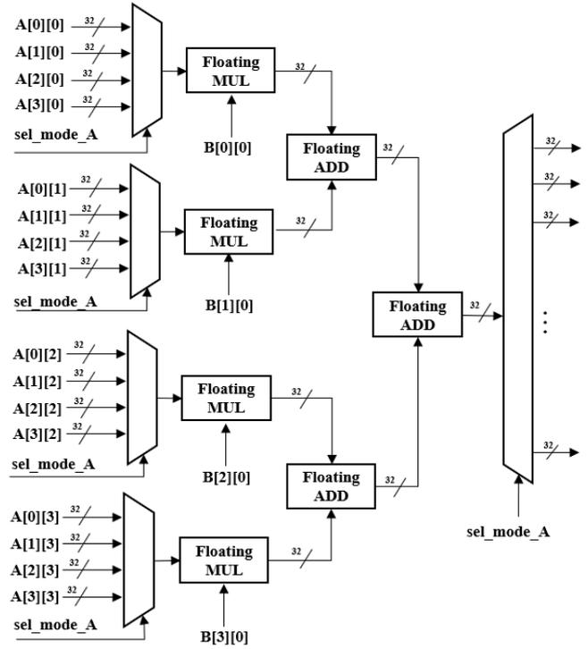
Fig. 4 Block diagram of a  $4 \times 4$  matrix multiplier by a  $4 \times 1$  matrix
