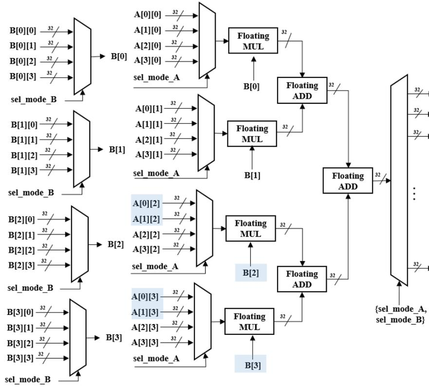
Fig. 3 Block diagram of a  $4 \times 4$  matrix multiplier by a  $4 \times 4$  matrix
