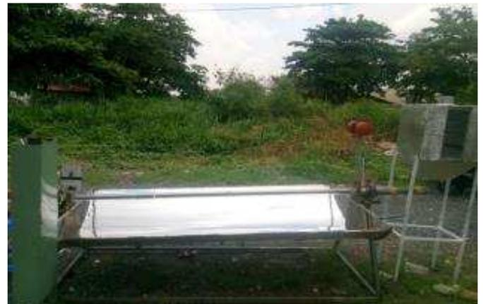
Fig. 6 The glass tube collector placed on the focus of a parabola surface.
