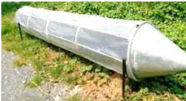
Fig. 4 Pipe collector covered by transparent polyethylene.
