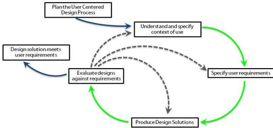
Fig. 3 Phases of UCD by ISO 9241 – 210 [32]
