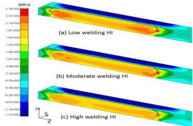
Fig. 7 Effect of change in heat input on weld line distribution [101]
