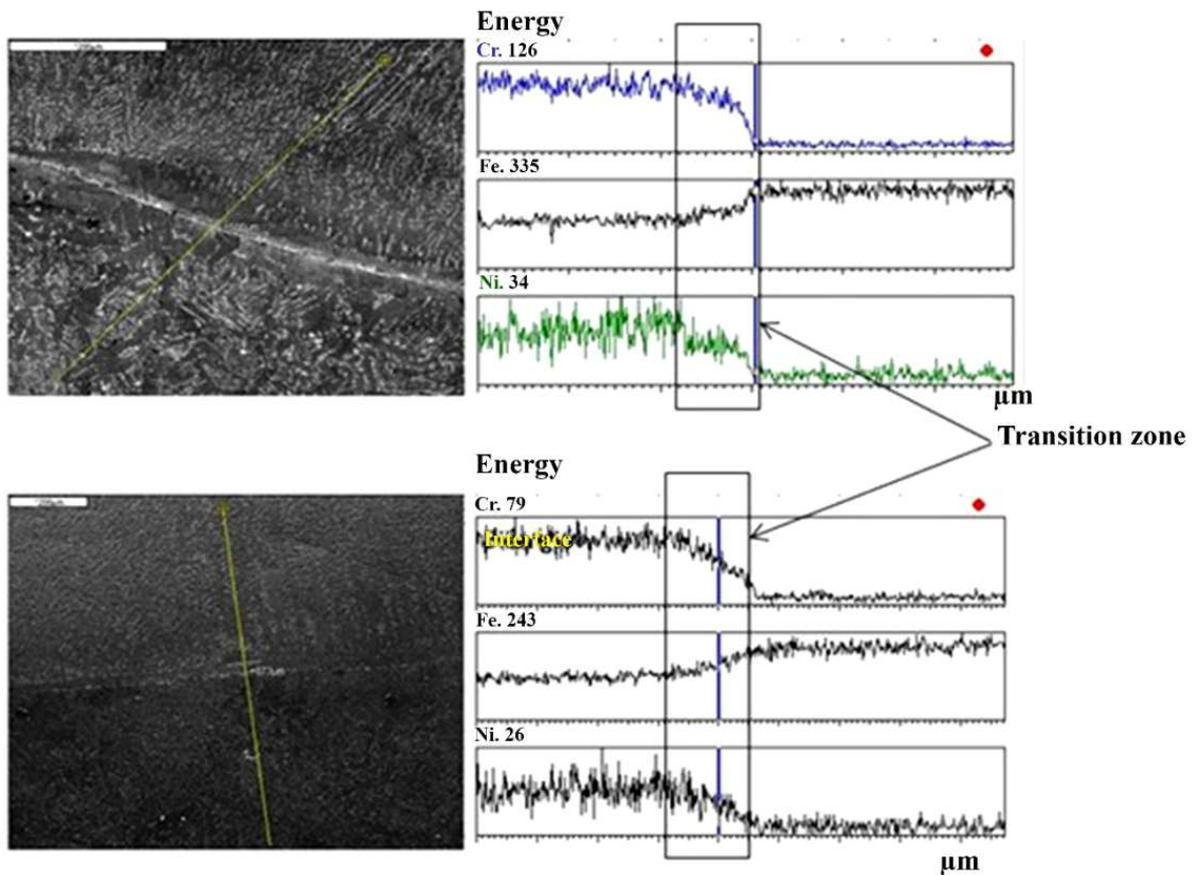
Fig. 3 Concentration distribution curves of elements in the transition zone [77]
