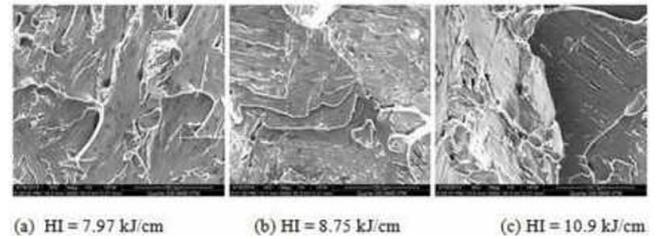
Fig. 9 SEM images of the weld deposition impact test surface under different heat inputs [103]
