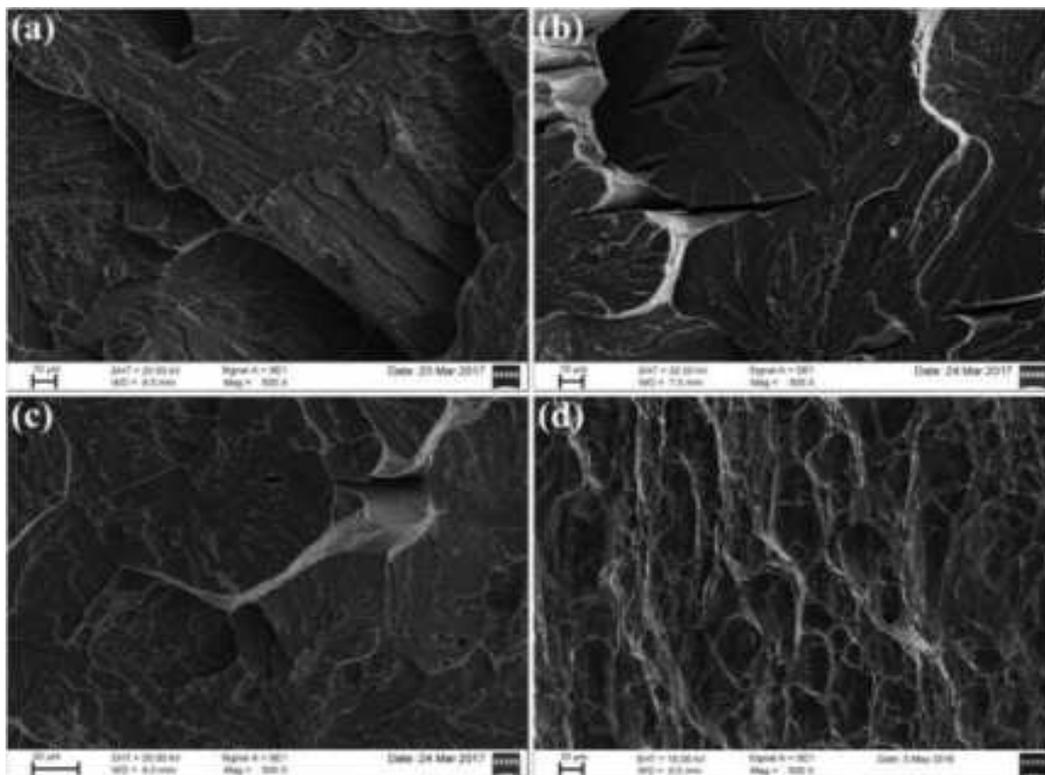
Fig. 11 SEM images of EB welds with different heat inputs of (a) 0.43, (b) 0.46, (c) 0.50 kJ/mm, and (d) BM [106]
