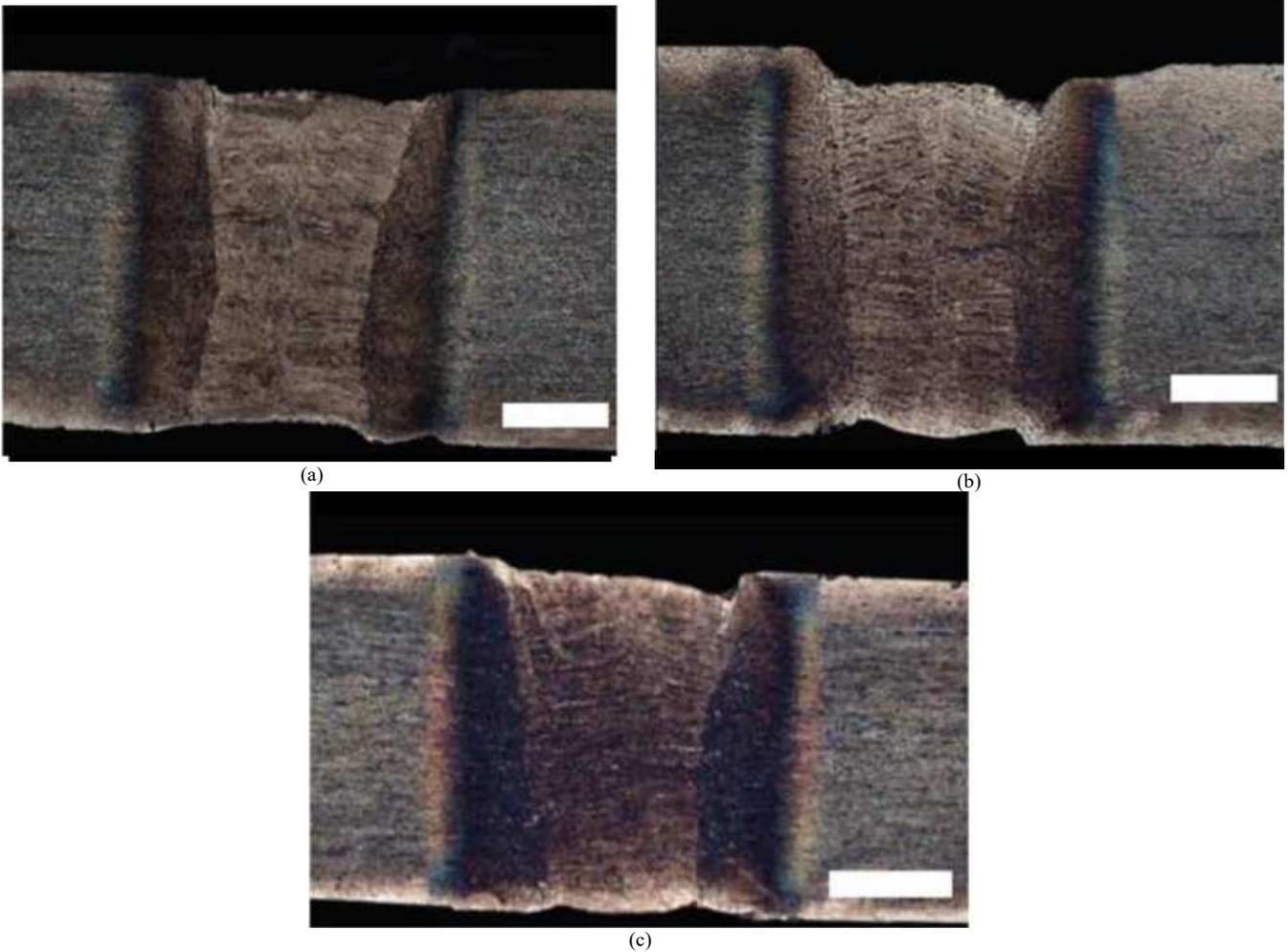
Fig. 10 Microstructure of the weld joint with a process heat input of 0.051 kJ/mm (a); 0.043 kJ/mm (b); 0.037 kJ/mm (c) [106]
