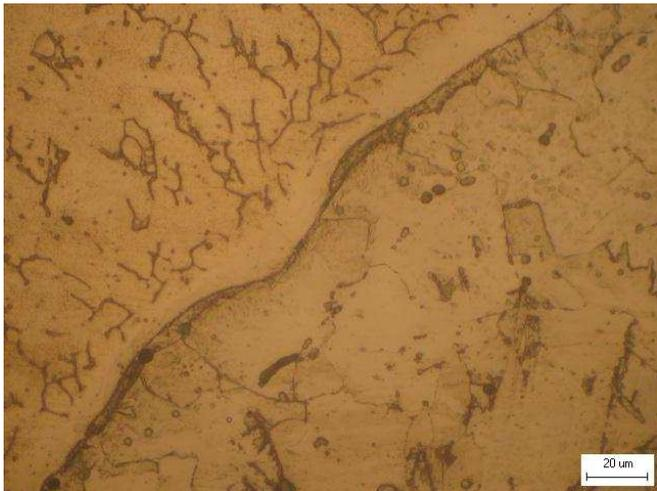
Fig. 5 Microstructure at carbon steel melting boundary (x500) [77]
