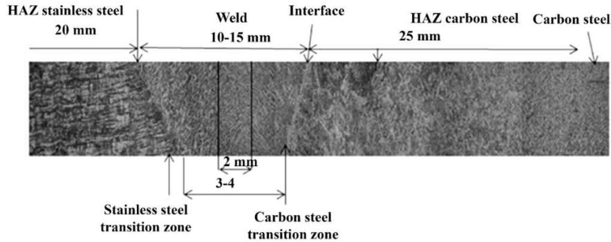
Fig. 2 Overview diagram of the structure of the weld between stainless steel and carbon steel [77]
