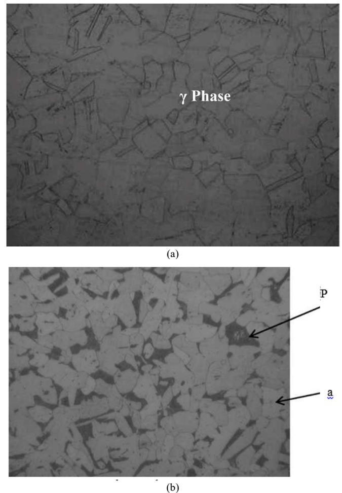
Fig. 1. a) Microstructure of stainless steel (x200); b) Microstructure of carbon steel (x200) [77]
