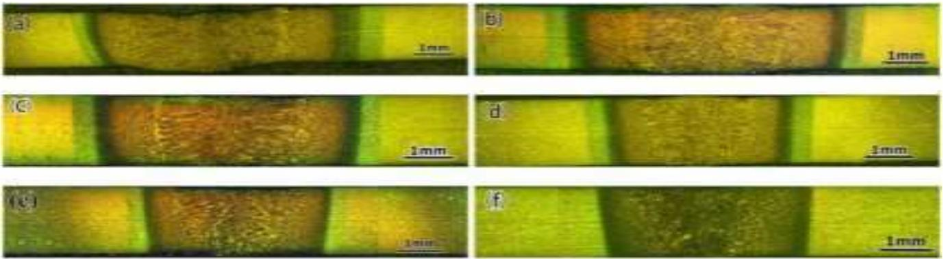
Fig. 8 Division of welding zone structure when (a) Input energy is 325 J/mm; (b) Input energy is 217 J/mm; (c) Input energy is 163 J/mm; (d) input energy is 130J/mm; (e) input energy is 108 J/mm and (f) input energy is 93 J/mm [102]
