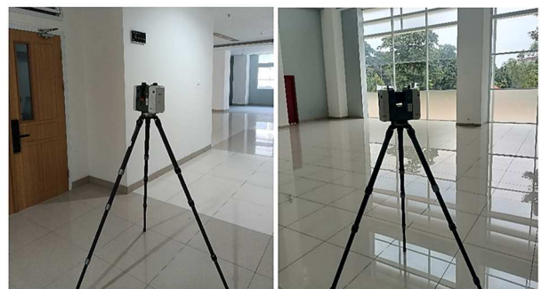
Fig. 2 Point cloud acquisition process (Source: Author Documentation)
