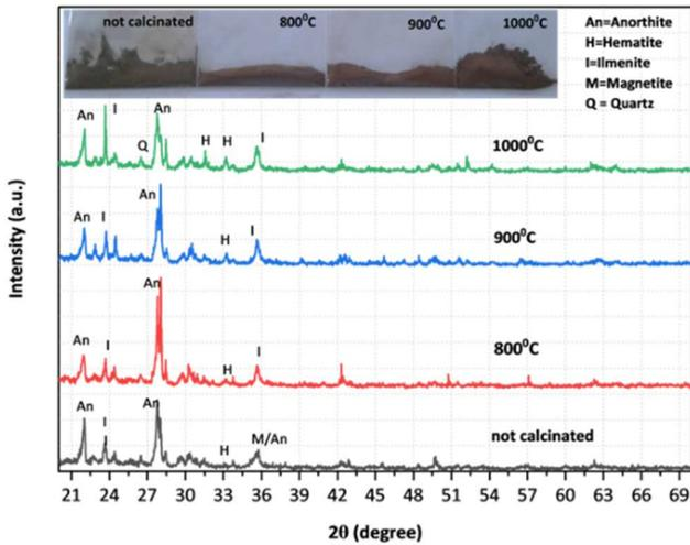
Fig. 4 XRD spectra of Lokon volcanic ash
