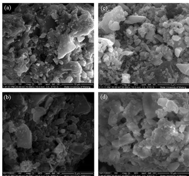
Fig. 7 SEM image of Lokon ash (a) not calcinated, (b) 800°C, (c) 900°C, (d) 1000°C
