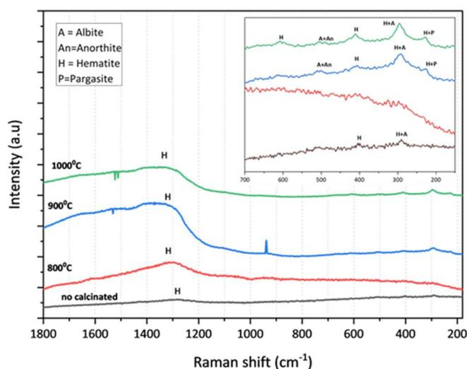
Fig. 3 Raman spectra of not calcinated and calcinated samples
