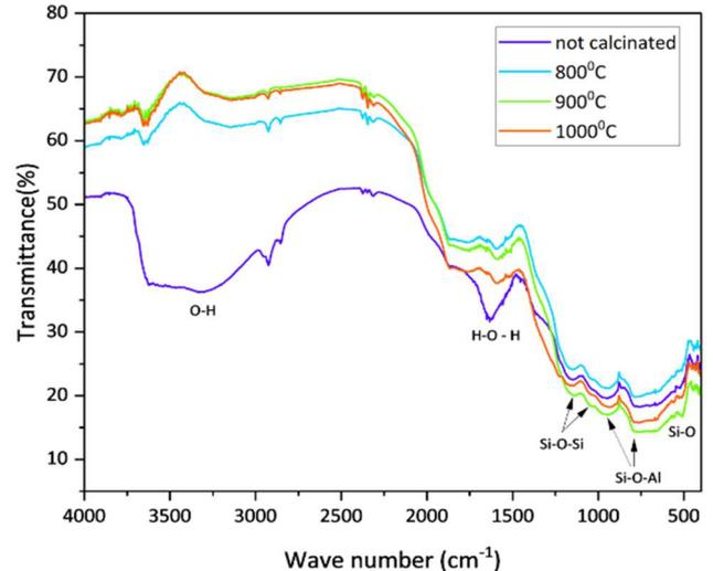
Fig. 6 FTIR spectra of volcanic ash
