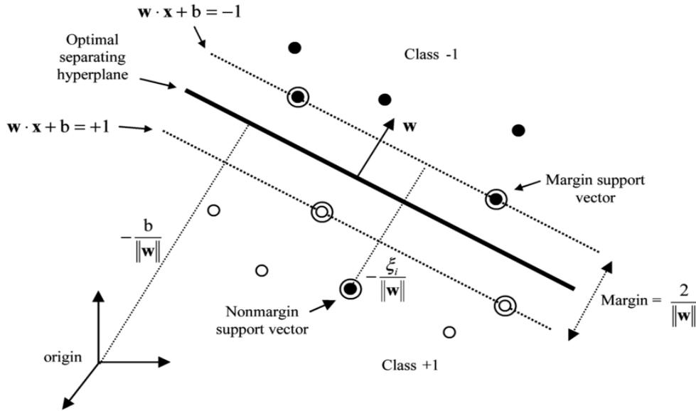
Fig. 4 Illustration of Support Vector Machines finds the optimal hyperplane [21]
