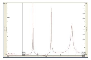
Fig 2. FRF for the first node of glass
