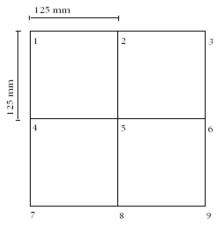
Fig 1. Specimen with nine nodes position on the plate surface
