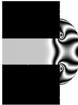
(a).  $x = 9.0 \text{ mm}$  and density fringe step 0.2.
