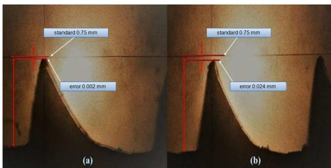
Fig. 5 The Comparison between the smallest and largest screw height errors under different machining conditions.
