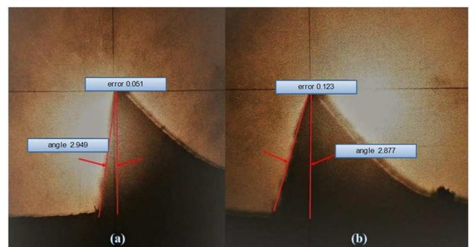
Fig. 7 The comparison between the smallest and largest screw angle error values  $\beta$  at different cutting conditions.
