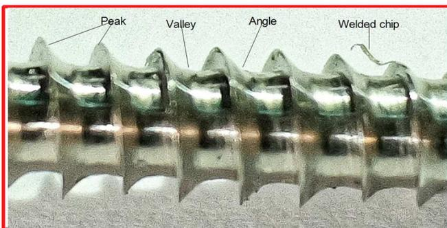
Fig. 8 Cortical Ti-6Al-4V ELI screw produced under optimal cutting conditions (spindle rotation speed of 100 rpm, depth of cut of 0.01 mm, and type of VCO lubricant)
