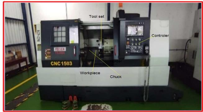
Fig. 1 CNC lathe machine used in this experiment of Feeler FTC-350XL type.
