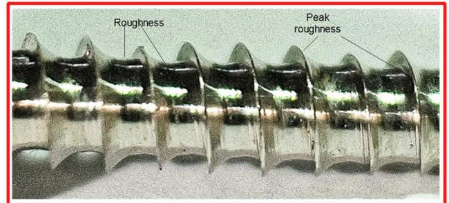
Fig. 9 Cortical Ti-6Al-4V ELI screw produced under cutting conditions with a spindle rotation speed of 100 rpm and a depth of cut of 0.03 mm
