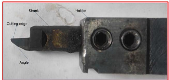
Fig. 2 Cortical cutting tool of carbide material used in cutting Ti-6Al-4V ELI.
