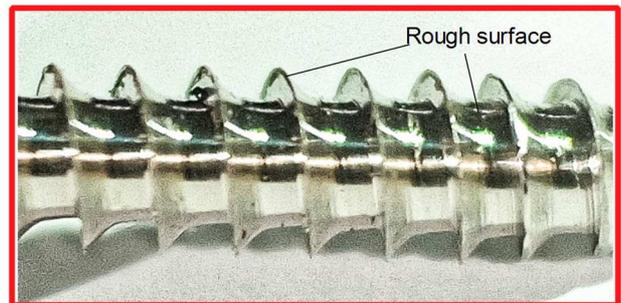
Fig. 11 Cortical Ti-6Al-4V ELI screw produced under cutting conditions with a spindle rotation speed of 300 rpm and a depth of cut of 0.03 mm.
