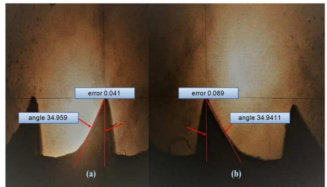
Fig. 6 The comparison between the smallest and largest screw angle errors  $\alpha$  at different cutting conditions.
