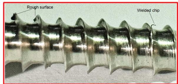
Fig. 10 Cortical Ti-6Al-4V ELI screw produced under cutting conditions with a spindle rotation speed of 200 rpm and a depth of cut of 0.03 mm
