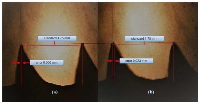
Fig. 4 The comparison between the smallest and largest screw peak errors at different machining conditions
