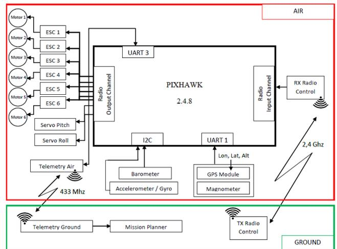
Fig. 1 UAV System Block Diagram
