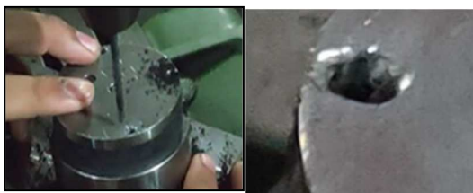
Fig. 3 The process of making holes using a drill and jig
