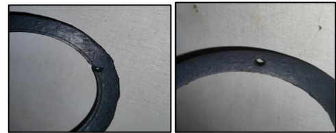
Fig. 4 NG gasket hole oval/elliptical/hole diameter less than 3mm
