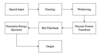
Fig. 4 Block Diagram of MFCC Feature Extraction
