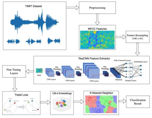
Fig. 1 Block Diagram of the Proposed Approach
