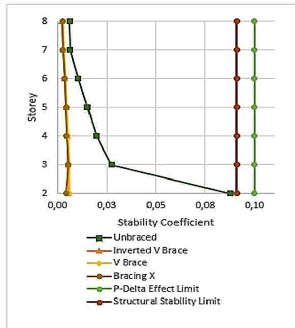
Fig. 11 P-Delta Effect for X Direction
