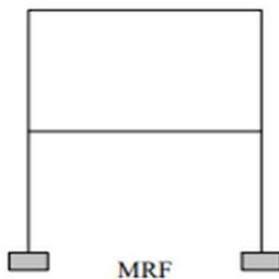
Fig. 1 Moment resisting system configuration frame (MRF)
