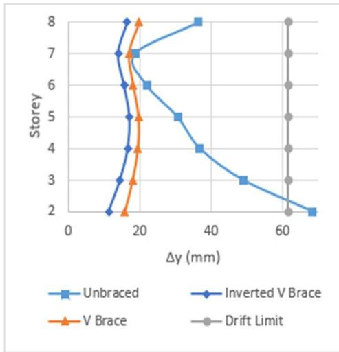
Fig. 10 Storey Drift for Y- direction
