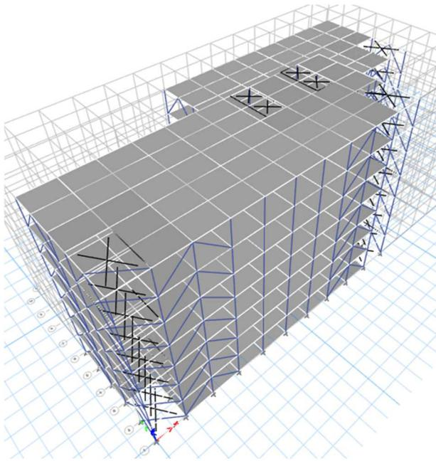
Fig. 7 Structure with Inverted V Bracing
