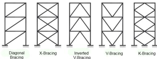
Fig. 2 Concentrically braced system configuration frame (CBF)
