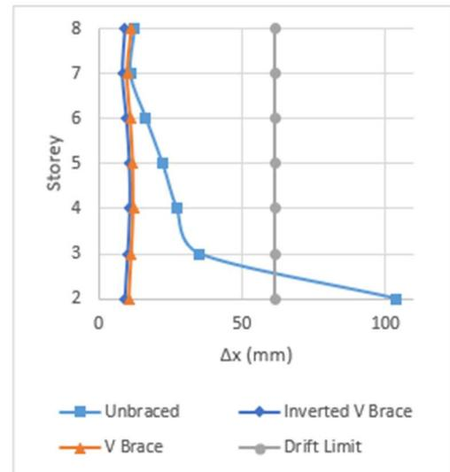
Fig. 9 Storey Drift for X-direction
