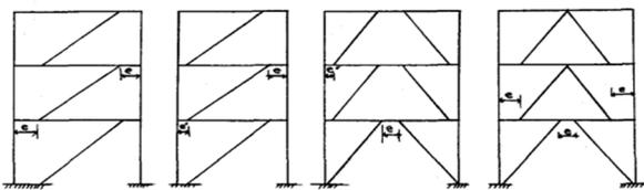
Fig. 3 Eccentrically braced system configuration frame (EBF)
