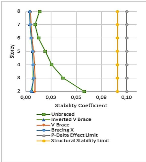
Fig. 12 P-Delta Effect for Y Direction
