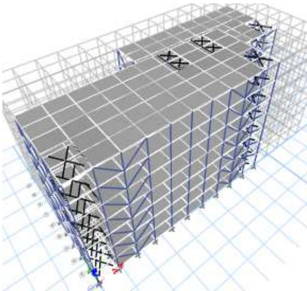
Fig. 8 Structure with V Bracing
