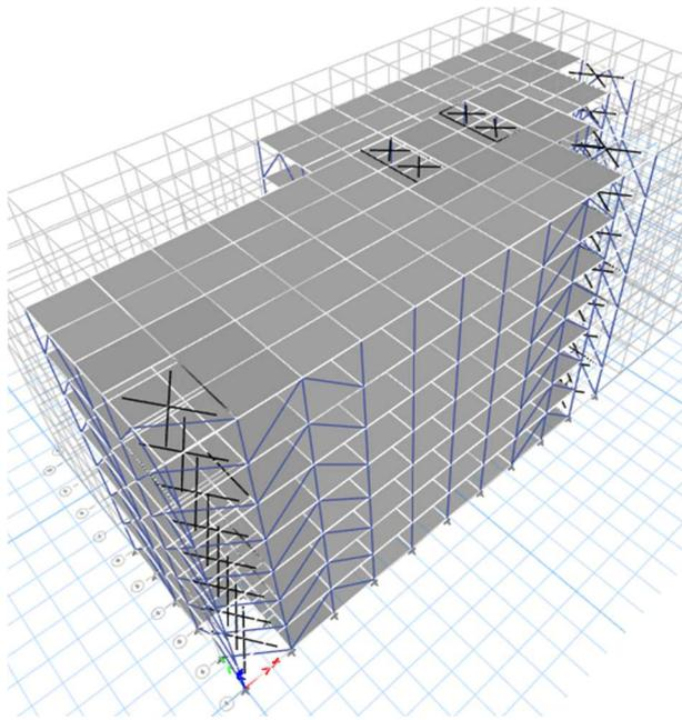
Fig. 7 Structure with Inverted V Bracing
