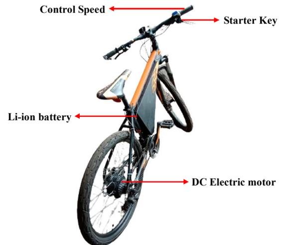
Fig. 1 Electric bicycle setup as an experimental system
