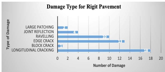
Fig. 6 Graph of Damage Types in Rigid Pavement
