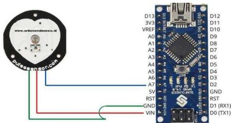
Fig. 4 Arduino-Nano Circuit Connected to Pulse Sensor
