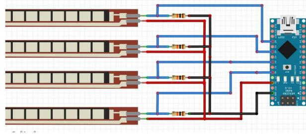
Fig. 1 Arduino-Nano with Flex Sensor
