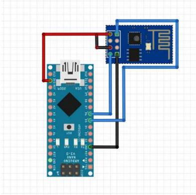
Fig. 3 Arduino-Nano with Modul WIFI ESP-01
