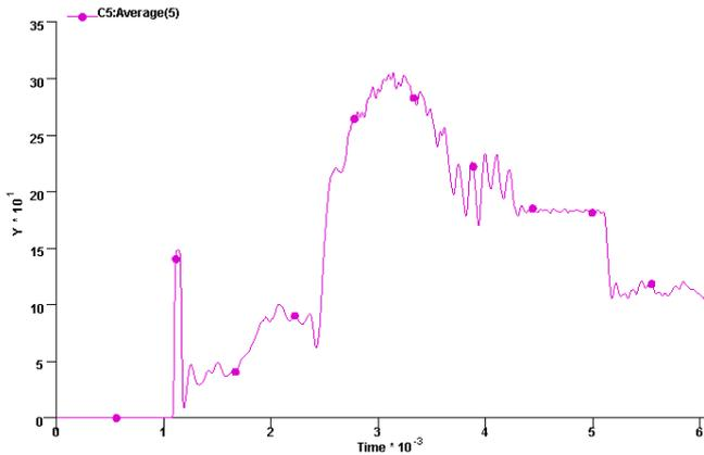
Fig. 11 Force graph of the deep drawing process
