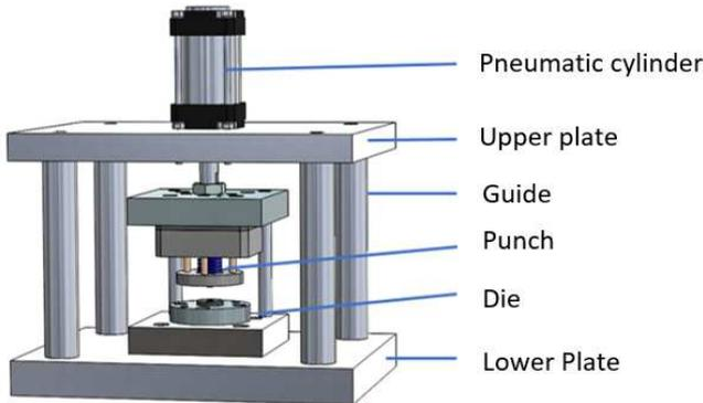
Fig. 6 3D model of connector head part stamping die set
