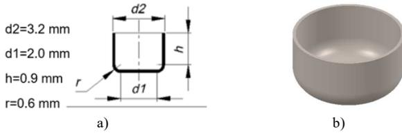
Fig. 2 Detailed geometrical parameters of the connector head: a) 2D product dimensions b) 3D product model
