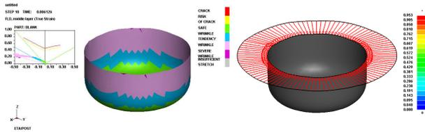
Fig. 9 Simulation results of wrinkles and tears of the product. a) Ability to create product shape; b) Ability to pull material into the die cavity
