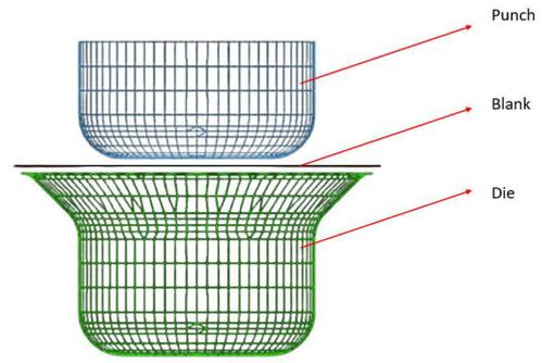
Fig. 7 The model assembly scheme in FEM
