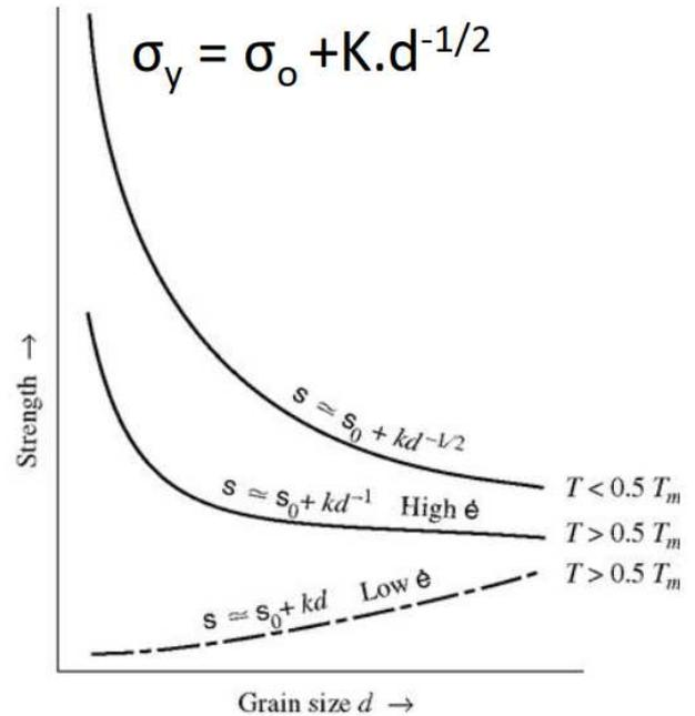
Fig. 4 Graph showing the correlation between grain size and tensile strength.
