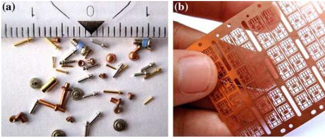
Fig. 1 Micro parts used in industry [4]: a) Massive forming of microscopic parts b) Stamping tiny parts from sheet metal billet.
