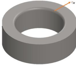
Fig. 5 3D model of drawing die
