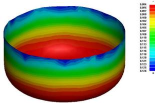
Fig. 10 Simulation results of thickness variation
