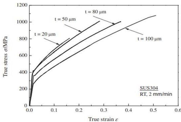
Fig. 3 Stress-strain curves of stainless steel sheets of different thickness [32]
