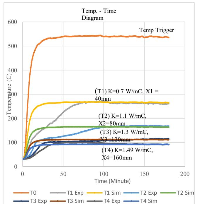
Fig. 5 Combined graph of experimental results and FEA simulation
