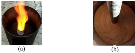
Fig. 1 (a) Syngas is produced by heating sawdust in the center of compacted sawdust on a bio stove (b) Saw dust in bio stove[24]
