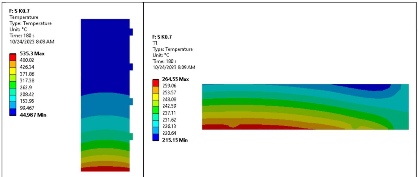
Fig. 9 Snapshot temperature distribution at each value  $k = 0.7$  of sawdust conductivity.
