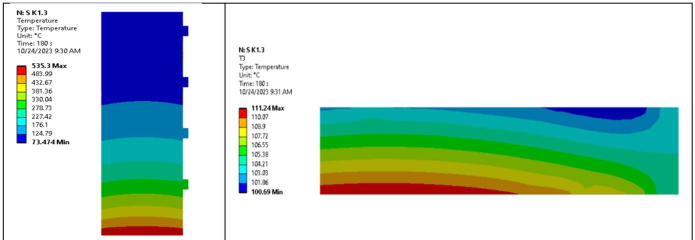
Fig. 7 Snapshot temperature distribution at each value k = 1.3 of sawdust conductivity.
