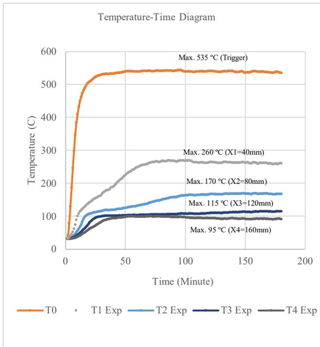
Fig. 4 Temperature, time graph, and illustration of experimental results
