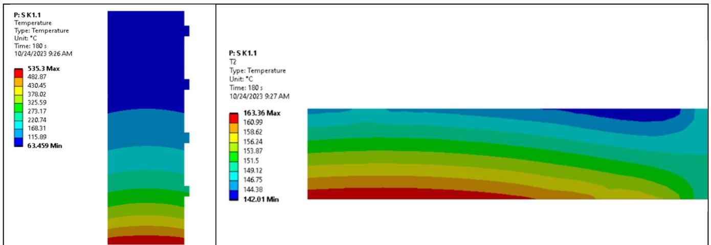
Fig. 8 Snapshot temperature distribution at each value k = 1.1 of sawdust conductivity.
