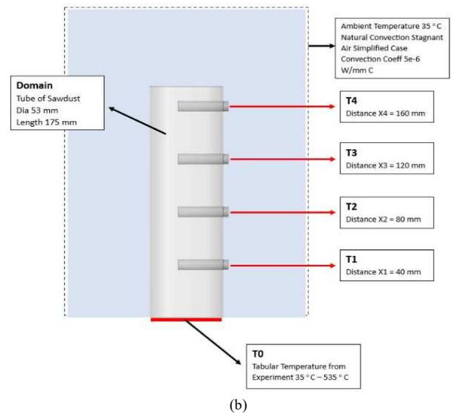
Fig. 2 (a) Experimental equipment to measure thermal effects during the pyrolysis process installed five thermocouples to measure compacted sawdust (b) FEA boundary conditions on compacted sawdust.
