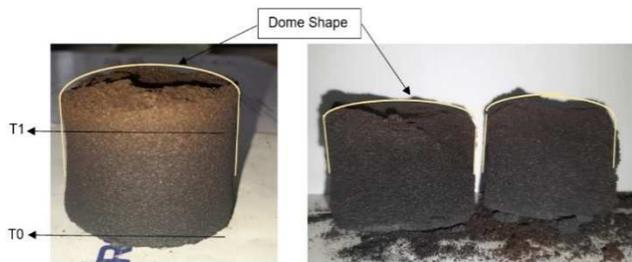
Fig. 10 Photo Sawdust Experiment Results after heating for 180 minutes.
