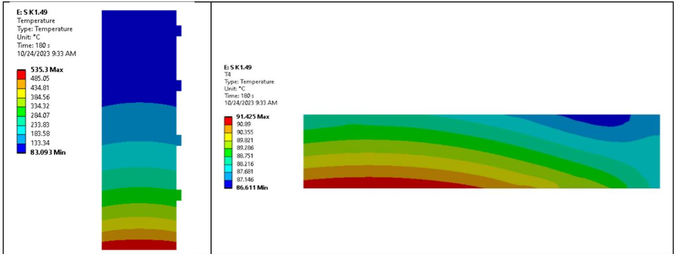
Fig. 6 Snapshot temperature distribution at each value k = 1.49 of sawdust conductivity
