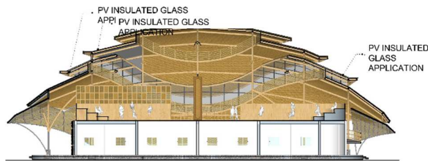
Fig. 9 Position of Alternative 1 PVIG in the building.
