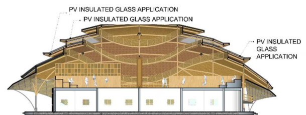
Fig. 14 An alternative position for 2 PVIG in the building.
