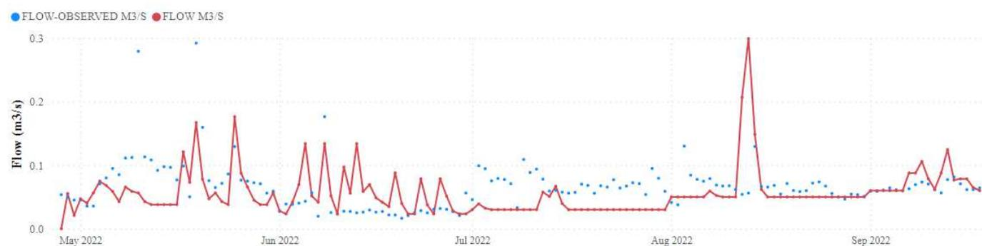
Fig. 3 The graph results simulating one sub-basin outflow and observed flow development from HEC HMS 4.11
