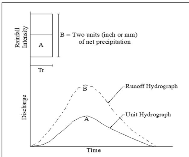
Fig. 2 The unit hydrograph derived from the runoff hydrograph
