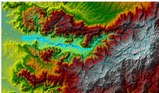
Fig. 4 The output of water depth values of Wiroko sub-watershed in HEC-RAS 2D unsteady flow hydrodynamics
