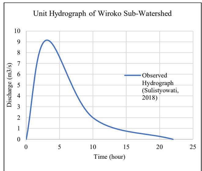
Fig. 3 Observed unit hydrograph of Wiroko sub-watershed [1]
