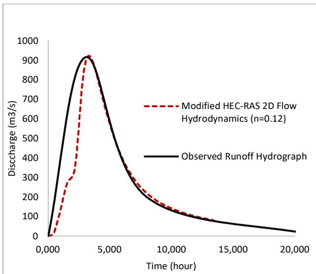
Fig. 6 The comparison between the observed runoff hydrograph and the modified HEC-RAS 2D numerical model hydrograph in the Wiroko sub-watershed
