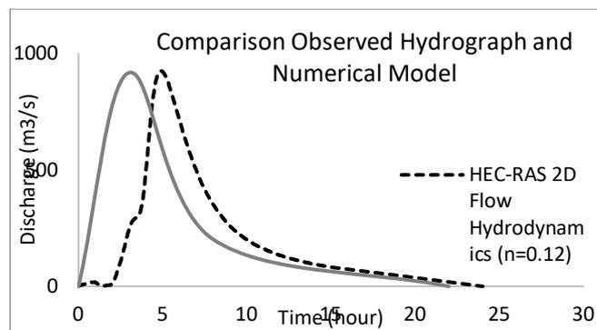
Fig. 5 The comparison results of the observed runoff hydrograph and HEC-RAS 2D numerical model hydrograph in the Wiroko sub-watershed
