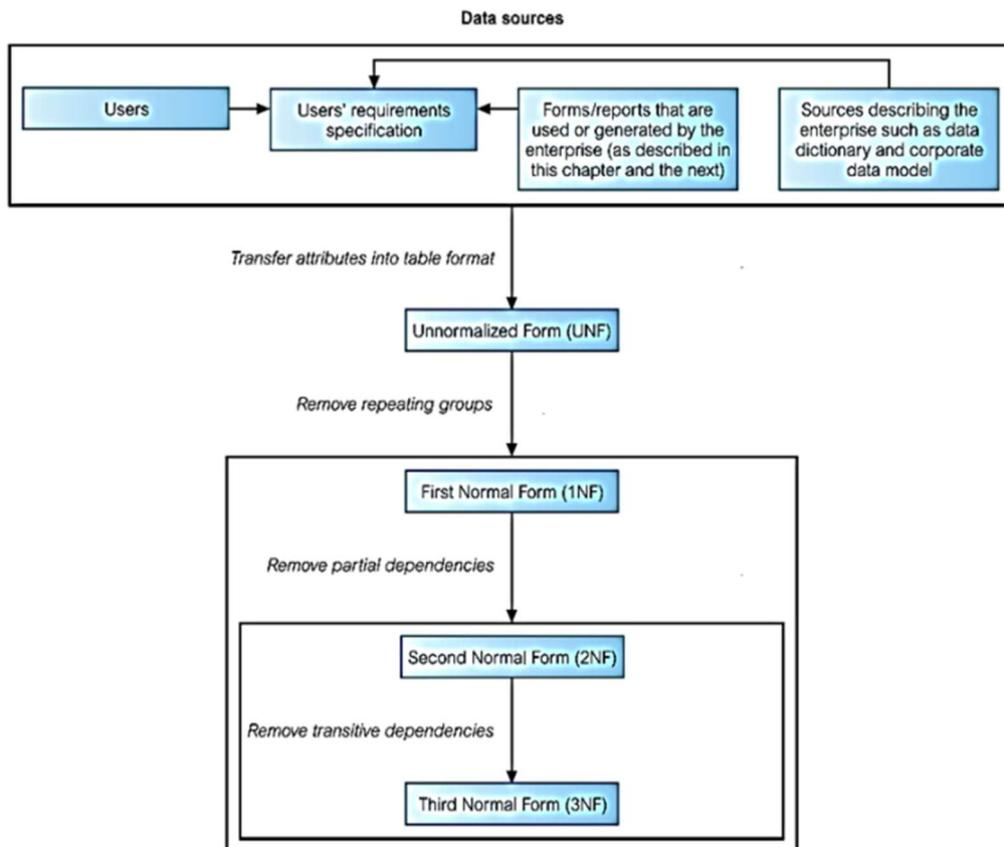
Fig. 2 Diagrammatic illustration of the process of normalization
