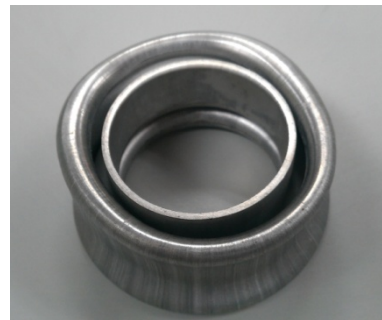
Fig. 13 Local buckling on Inversion tube: Top view
