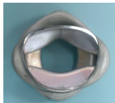
Fig. 14 Diamond shaped buckling
