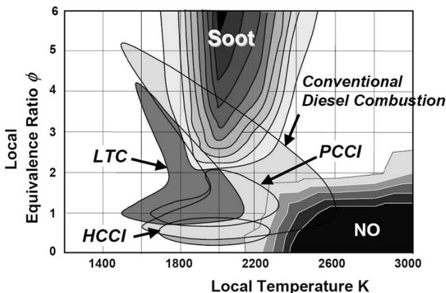
Fig. 2 NO<sub>x</sub> and soot formation in the relationship between temperature and equivalence ratio for diesel engine, PCCI, and HCCI mode [102]
