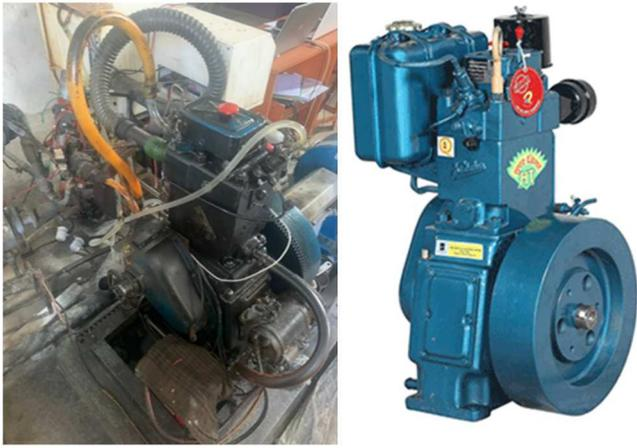
Fig. 3 Kirloskar TV1 engine for simulation
