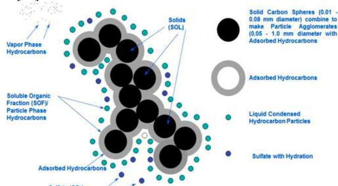
Fig. 1 PM formation process and components of PM [76]
