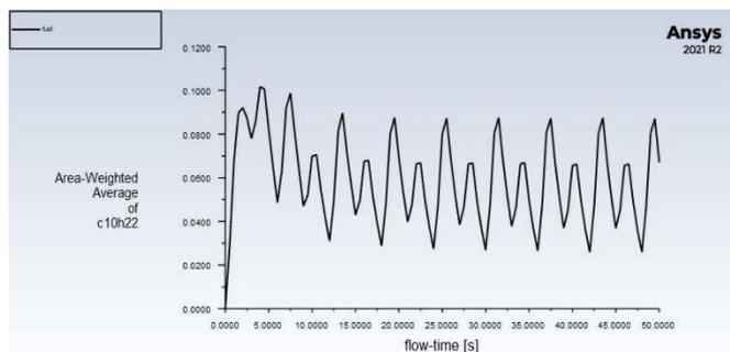
Fig. 6 Mass fraction of diesel fuel burnt in cylinder
