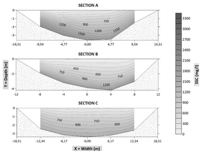
Fig. 6 The SSC was observed from Sec. A to Sec. C
