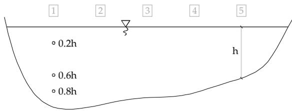
Fig. 4 Data collection points (0.2h, 0.6h, 0.8h) on five water-column in the river cross-sections
