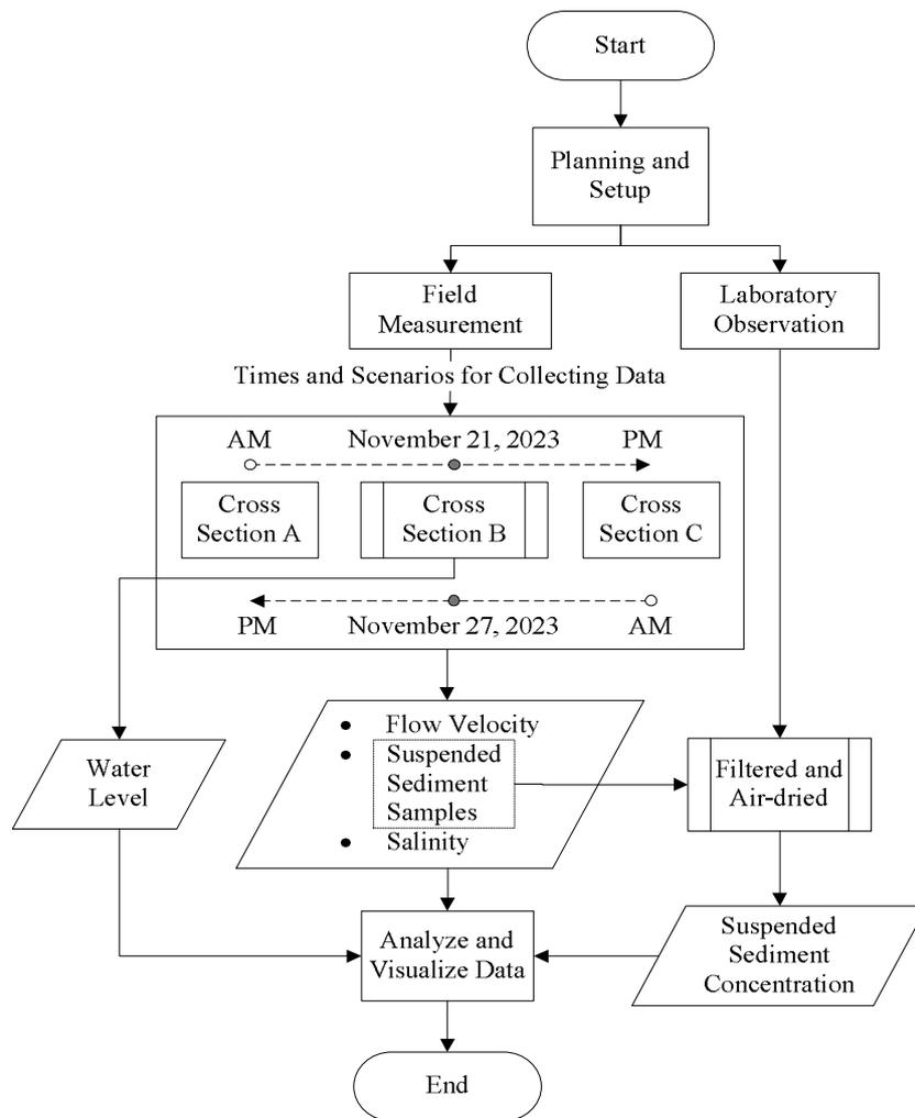
Fig. 1 Field and Laboratory Data Collection Process
