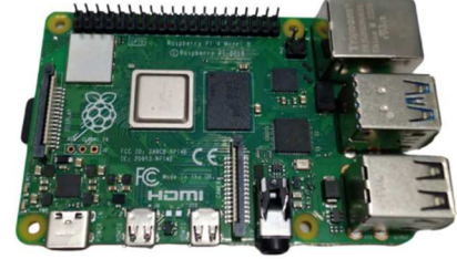
Fig. 4 An embedded microcomputer Raspberry Pi 4B where we implement our trained model
