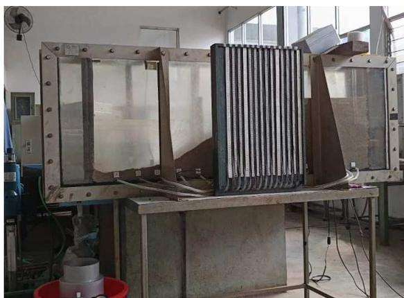
Fig. 4 Sand structure in permeability tank
