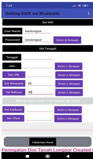
Fig. 12 Setting Early Warning System (EWS) application to set a threshold of alarm
