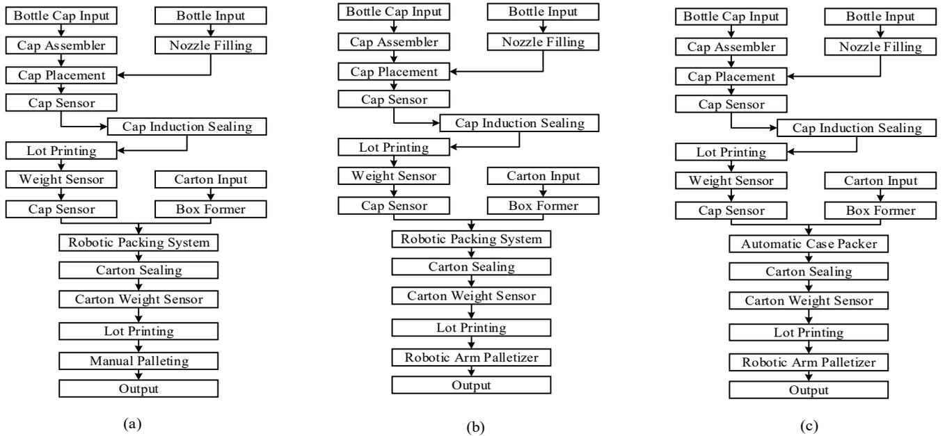
Fig. 3 Working diagrams for the three improvement scenarios: (a) Robotic Packing System, (b) Robotic Packing with Palletizer, and (c) Automatic Case Packer with Palletizer.
