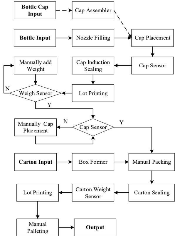
Fig. 2 Process Diagram for Line Filling and Packing
