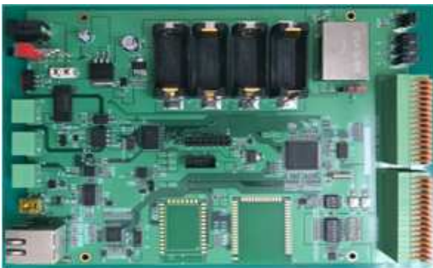
Fig. 2 The sensor node hardware board
