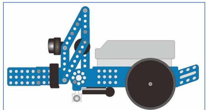
Fig. 1 Differential Wheel Robot Car with Arm
