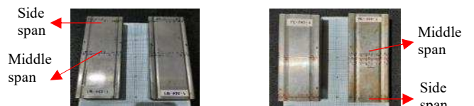
Fig. 23 The uncoating result for CFS lipped channel specimens
