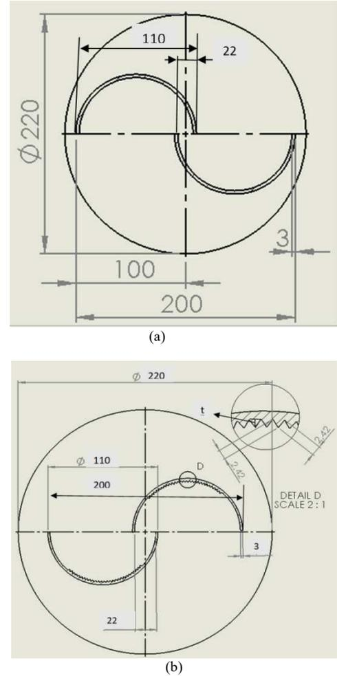
Fig. 1 Dimension (in mm) of Savonius models: a) conventional rotor b) rotor with zigzags of different heights
