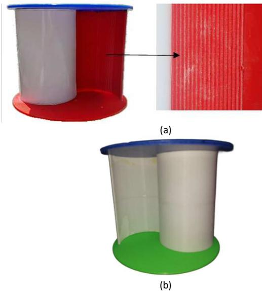
Fig. 2 (a) Zigzag model, (b) Semi-circular model
