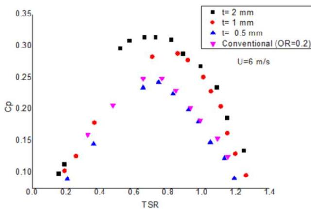
Fig. 6 Comparison of  $C_p$ - $TSR$  for variation of Savonius rotors
