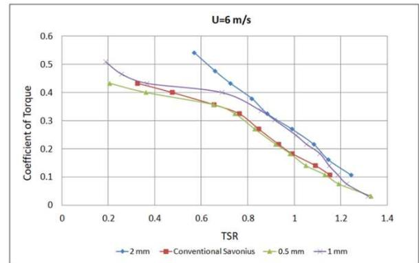
Fig. 7 Comparison of  $C_T$ - $TSR$  curves for models tested at speed of 6 m/s
