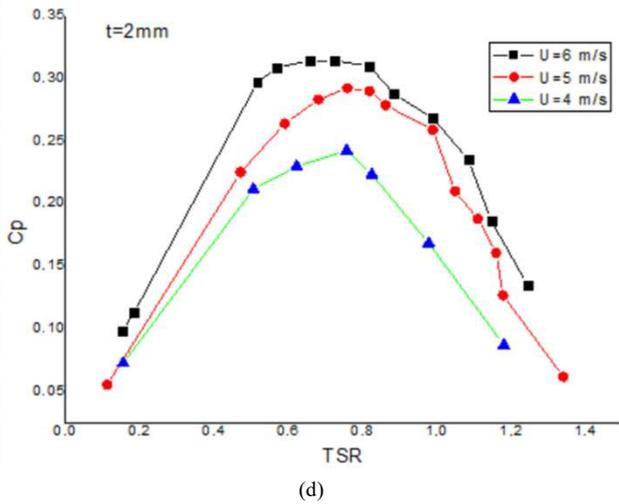
Fig. 5 Characteristics of  $C_p$ - $TSR$  at various inlet velocities for models tested: (a) conventional, (b)  $t=0.5$ mm, (c)  $t=1$ mm and (d)  $t=2$ mm
