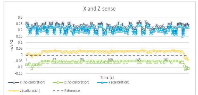
Fig. 9 (c) X and Z-sense at -Y-axis (g)
