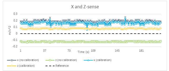
Fig. 9 (a) X and Z-sense at +Y-axis (g)
