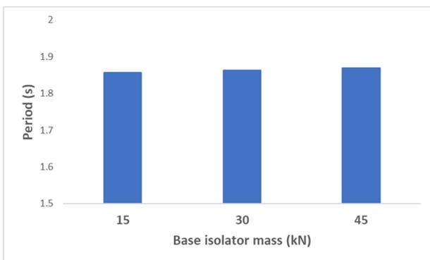
Fig. 5 Building period for Different Base Isolator Masses
