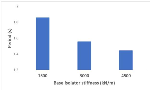
Fig. 8 Building period for Different Base Isolator Stiffness
