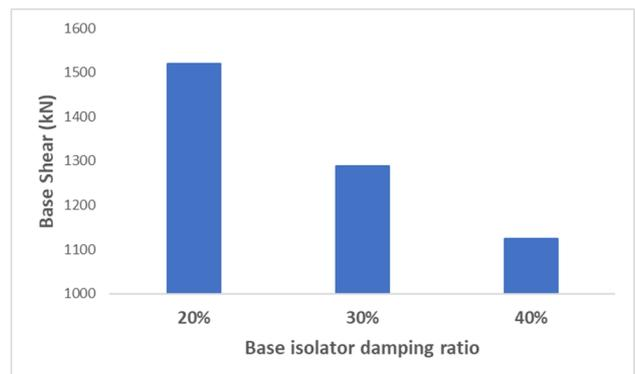
Fig. 10 Base Shear for Different Base Isolator Damping Ratio
