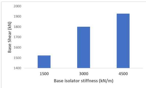
Fig. 7 Base Shear for Different Base Isolator stiffness
