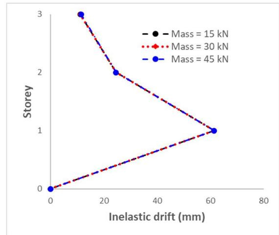
Fig. 6 Inelastic storey drift for Different Base Isolator Masses
