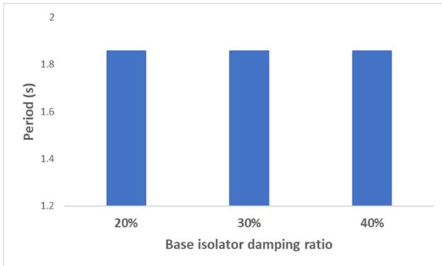
Fig. 11 Building period for Different Base Isolator Damping Ratio
