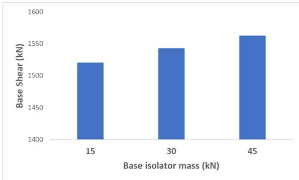
Fig. 4 Base Shear for Different Base Isolator Masses
