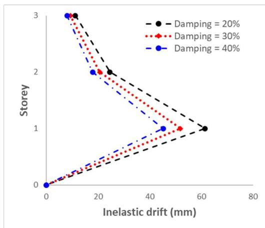
Fig. 12 Inelastic storey drift for Different Base Isolator Damping Ratio
