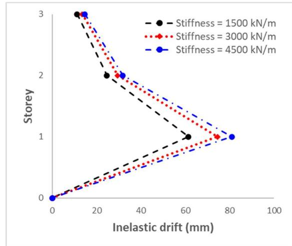
Fig. 9 Inelastic storey drift for Different Base Isolator Stiffness
