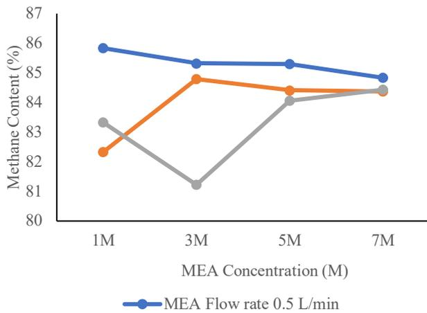
Fig. 6 The effect of MEA flow rate on the CH<sub>4</sub> produced
