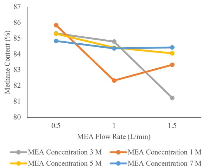
Fig. 5 The effect of flow rate on the CH<sub>4</sub> produced
