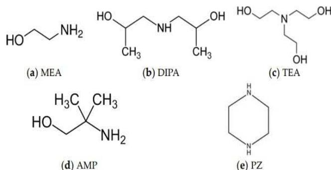
Fig. 2 Structure of Various Amines [2]
