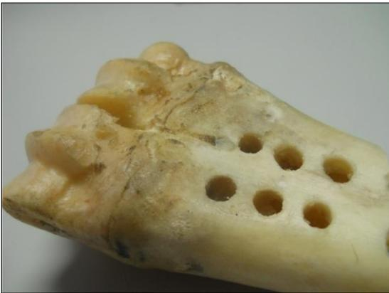
Fig. 6 Drilled location of cow bone (tibia)
