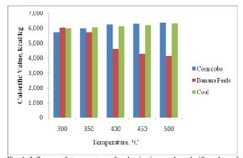
Fig. 1 Influence of temperature of carbonization on the calorific value of carbonized corn cobs, carbonized banana peels and carbonized fine coal waste
