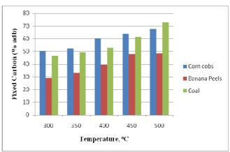
Fig. 5 Influence of temperature of carbonization on the fixed carbon of carbonized corn cobs, carbonized banana peels and carbonized fine coal waste
