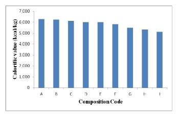
Fig. 6 Influence of carbonized corn cobs, carbonized banana peels and carbonized fine coal waste composition (%w/w) on calorific value of biobriquette
