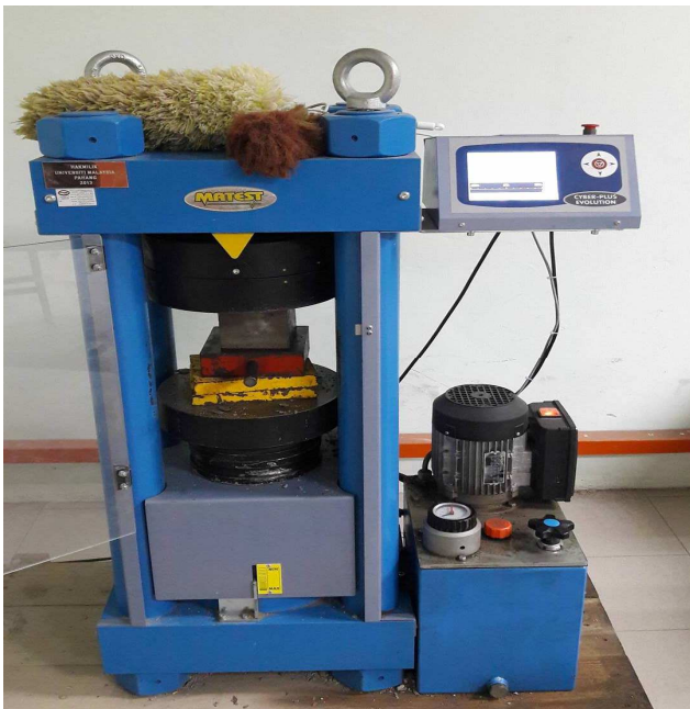
Fig. 3 Compression machine MATEST to perform compressive strength test on concrete cube specimens
