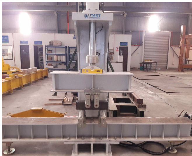
Fig. 4 Universal Testing Machine to perform flexural strength test on concrete beam specimens
