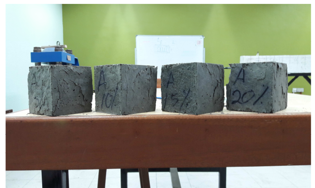
Fig. 9 Eggshell concrete cube specimens after undergo compressive strength test
