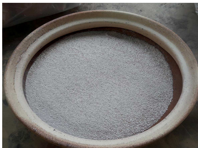
Fig. 2 Air dried eggshell powder after grinding process
