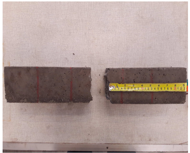
Fig. 12 Eggshell concrete beam specimens after undergo flexural strength test
