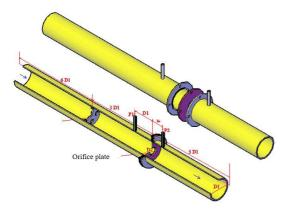
Fig. 3: Schematic diagram of the orifice plate
