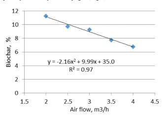
Fig. 9. Effect of air-flow on the biochar
