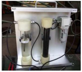
Fig. 2. The gasboard 3100P syngas analyzer
