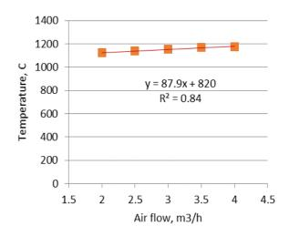
Fig. 4. Effect of air-flow on the syngas temperature
