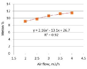
Fig. 7. Effect of air-flow on Methane
