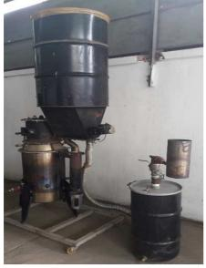
Fig. 1b. The downdraft gasifier
