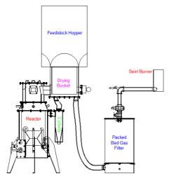
Fig. 1a. Schematic diagram of downdraft gasifier
