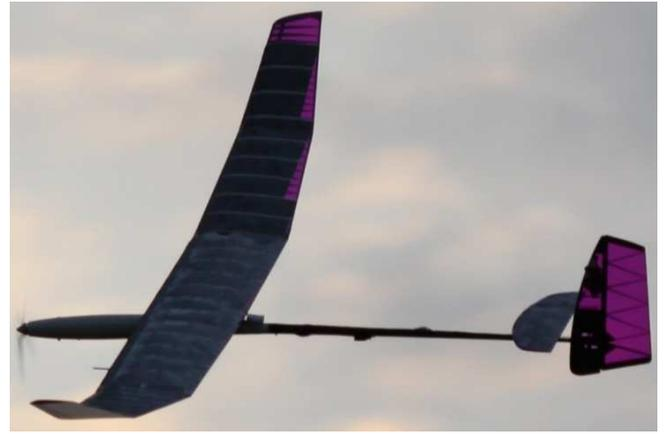
Fig. 2 Solar-powered UAV developed Aircraft Design Group, Cranfield University
