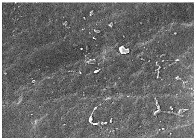
Fig. 3. Surface structure of the CA membrane 18% dope solution at room temperature at 5000x magnification
