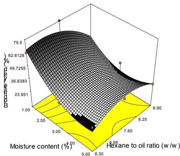
Fig.3. Combined effect of moisture content of jatropha seed and hexane to oil weight ratio on yield of biodiesel
