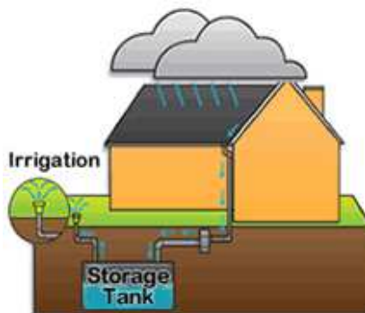
Fig 1. Rainwater Harvesting System for Irrigation
