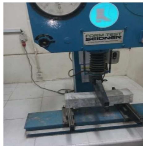
Fig. 8 Flexural test on beam
