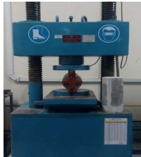
Fig. 7 Splitting tensile test on cylinder
