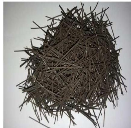
Fig. 4 The 1 inch length of steel fiber extracted from waste tyre
