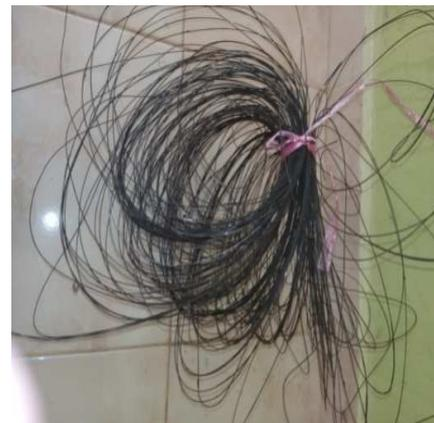
Fig. 3 Steel fiber extracted from waste tyre
