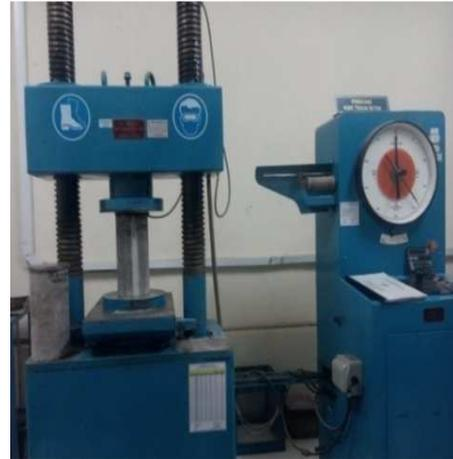
Fig. 6 Compressive test on cylinder
