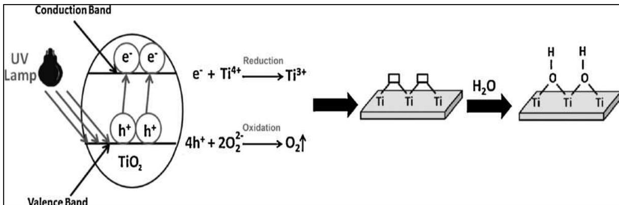
Fig. 1 Mechanism of TiO<sub>2</sub> hybrid on the substrate surface [12]
