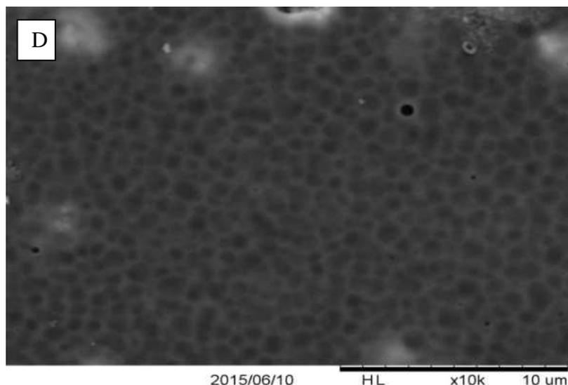
Fig. 3 SEM images of A) Polysulfone B) Polysulfone-PVP C) Polysulfone-TiO<sub>2</sub> D) Polysulfone-PVP-TiO<sub>2</sub> membranes under 10k magnification
