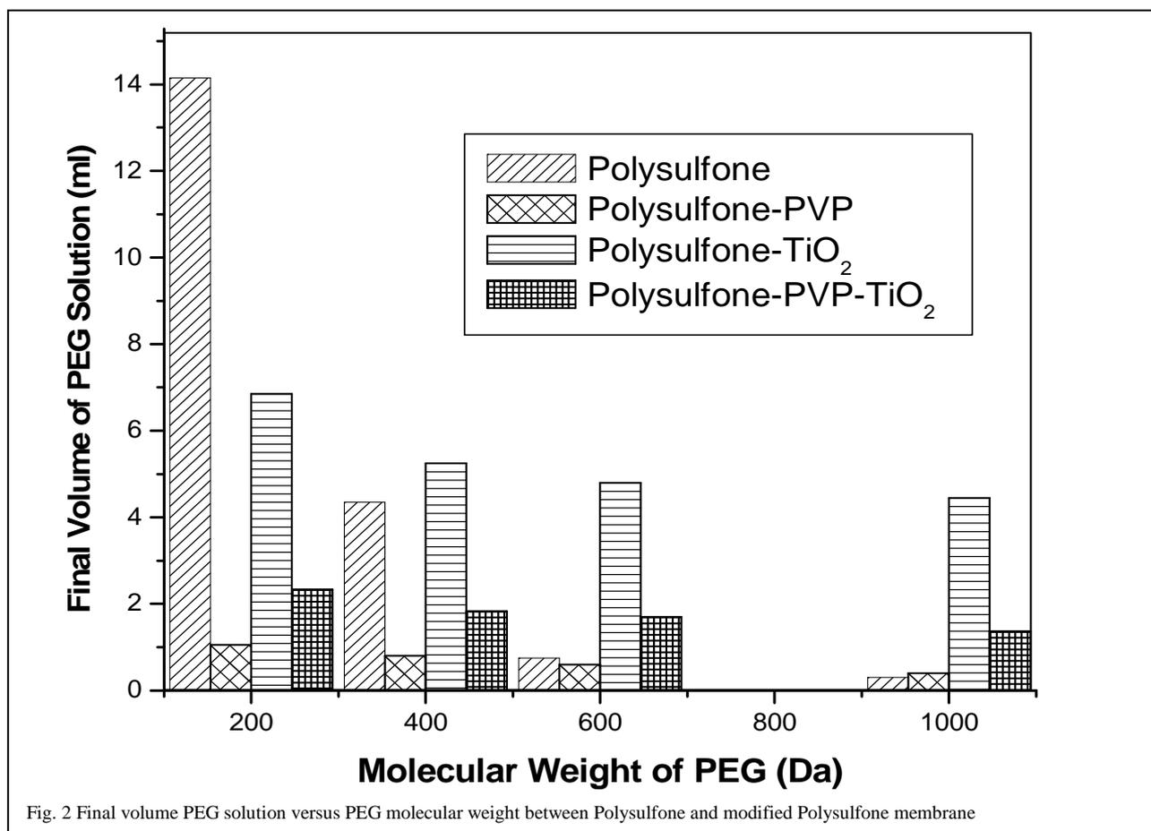
Fig. 2 Final volume PEG solution versus PEG molecular weight between Polysulfone and modified Polysulfone membrane
