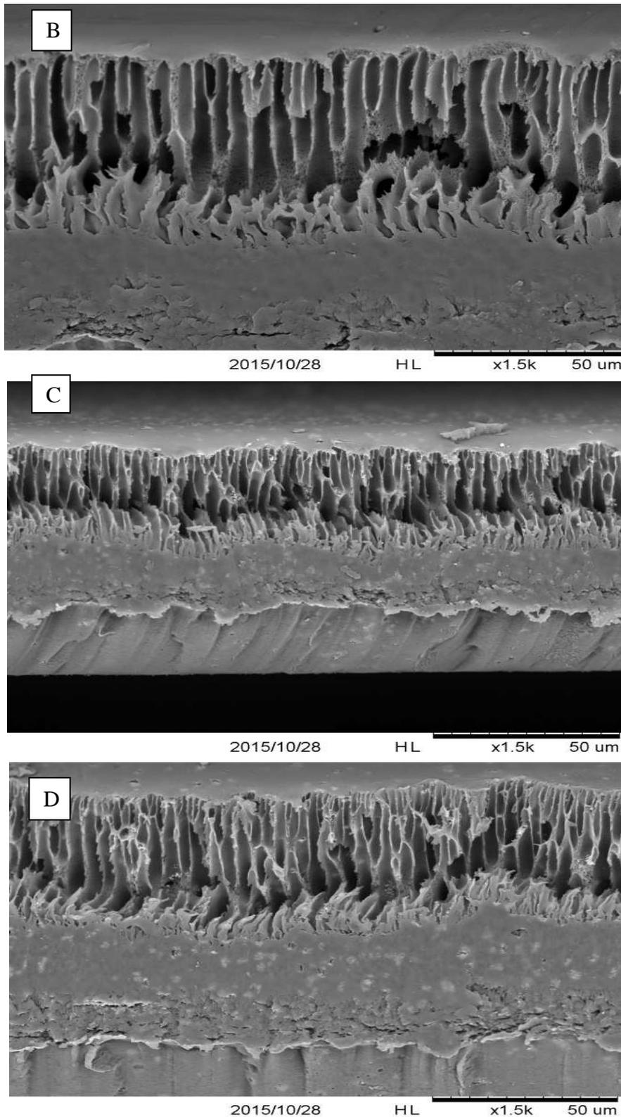
Fig. 4 SEM images of A) Polysulfone B) Polysulfone-PVP C) Polysulfone-TiO<sub>2</sub> D) Polysulfone-PVP-TiO<sub>2</sub> membranes under 1.5k magnification
