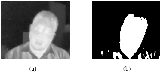
Fig. 3 Face Segmentation Based on Temperature; (a) Original Image, (b) Segmented face based on Temperature
