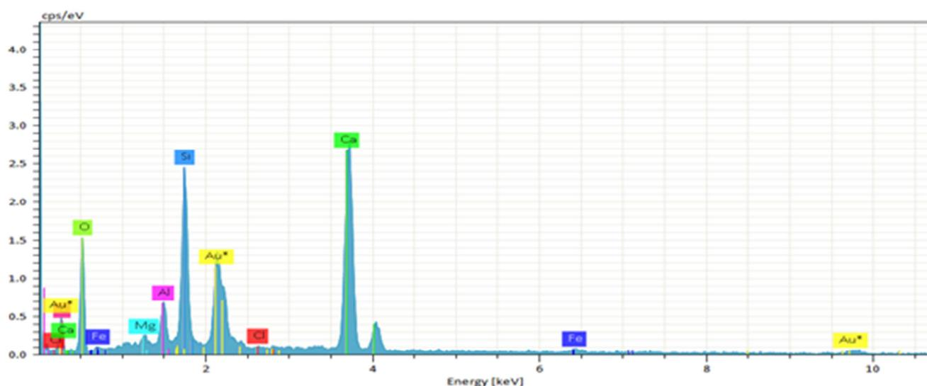
Fig. 13 EDX spectrum analysis of Kenaf Fibrous Concrete (KFC)
