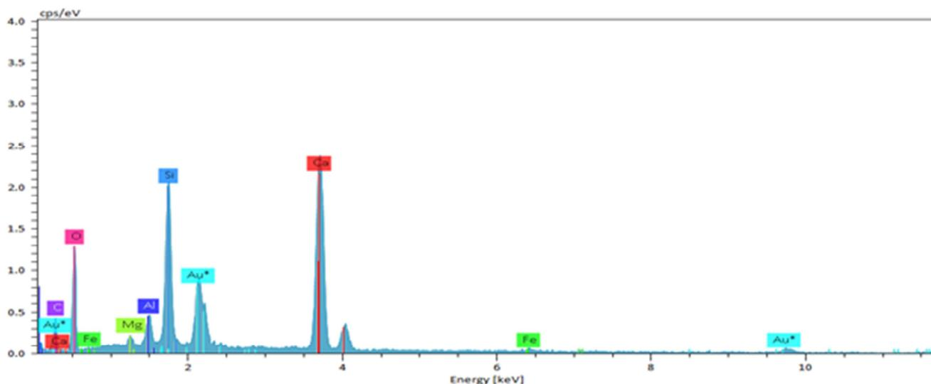
Fig. 12 EDX spectrum analysis of Normal Concrete
