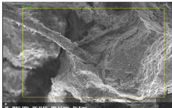
Fig. 11 SEM micrograph of Kenaf Fibrous Concrete (KFC)
