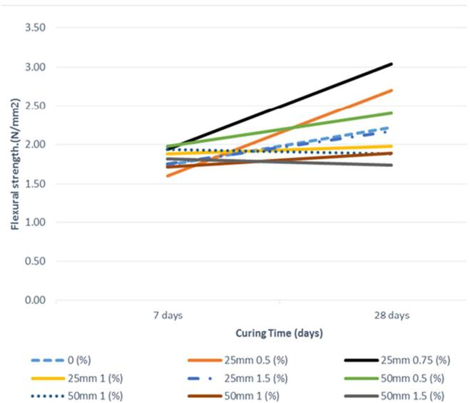
Fig. 7 Flexural Strength of Kenaf Fibrous Concrete (KFC)
