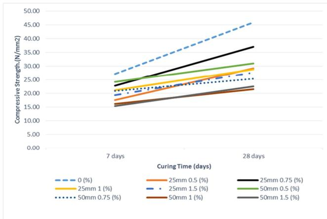
Fig. 5 Compressive Strength of Kenaf Fibrous Concrete (KFC)
