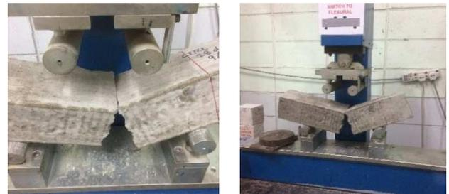
Fig. 8 Cracking failure of Control concrete
