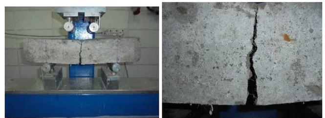
Fig. 9 Cracking failure of Kenaf Fibrous Concrete (KFC)
