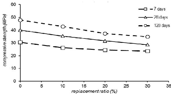
Fig. 4 Compressive Strength of R1, R2, and R3
