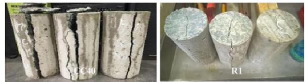
Fig. 10 Tensile crack patterns of CC40 and R1 in 28 days
