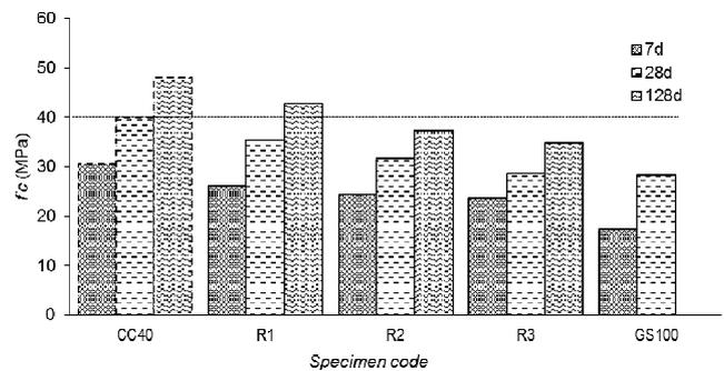
Fig. 6 Compressive strength of modified concrete
