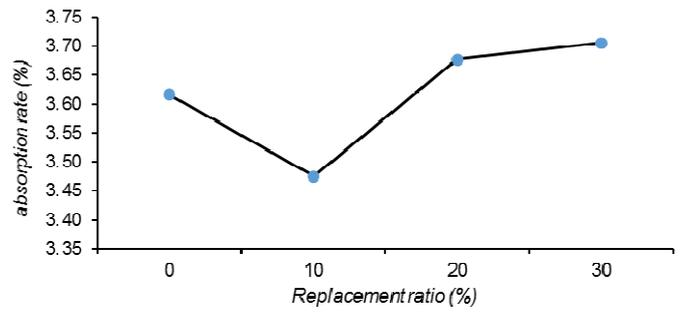
Fig. 13 Absorption rate of R1, R2, and R3
