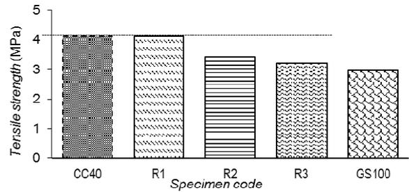
Fig. 9 Tensile strength of modified concrete in 28 days
