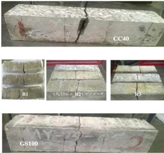
Fig. 12 Flexural crack patterns in 28 days
