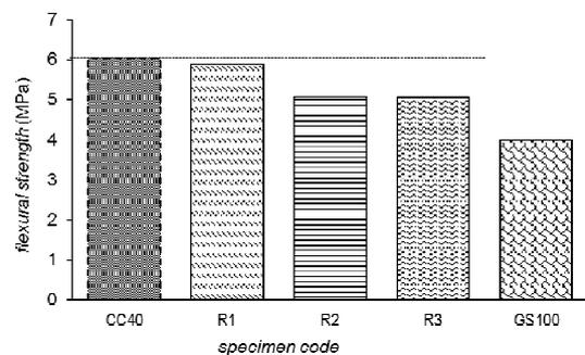
Fig. 11 Flexural strength of modified concrete in 28 days
